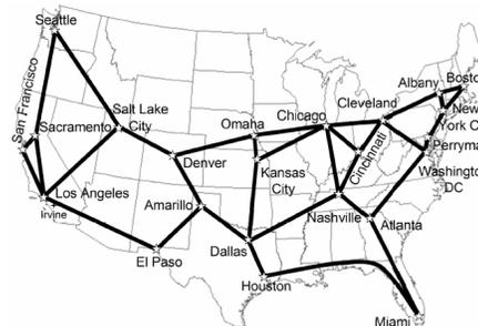
Fig. 3 Level 3 ISP backbone network in U.S.
